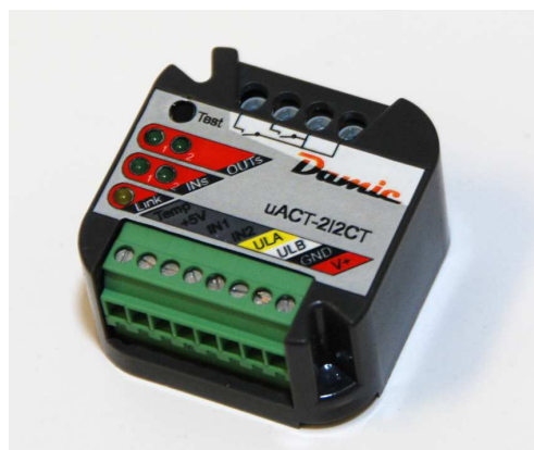
FIGURE 4: uACT 2i2ct – uLan Actuator and Temperature Sensor
